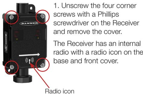
1. Unscrew the four corner screws with a Phillips screwdriver on the Receiver and remove the cover.
