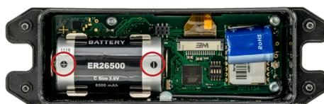
2. Insert the 3.6 V lithium battery. Verify the battery's positive and negative terminals align to the positive and negative terminals as marked.
