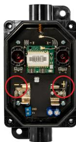
2. Insert the 3.6V lithium D cell battery. Verify the battery's positive and negative terminals align to the positive and negative terminals as marked.
