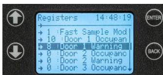
Repeat these steps for each additional door. By default, the **Fast Sample** setting is set to 1. This allows for change of state reporting. Change the **Fast Sample** setting to 0 to disable change of state reporting and increase the battery life.
