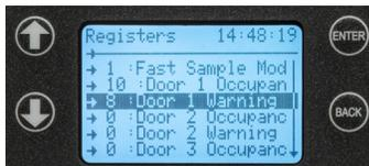
Repeat these steps for each additional door. By default, the **Fast Sample** setting is set to 1. This allows for change of state reporting. Change the **Fast Sample** setting to 0 to disable change of state reporting.
