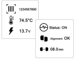
In-Series Diagnostics provides an array of additional data points for each In-Series Device used, including a unique tag value, internal temperature, voltage, and more, along with device-specific details such as the alignment and distance between a safety switch's sensor and actuator.
