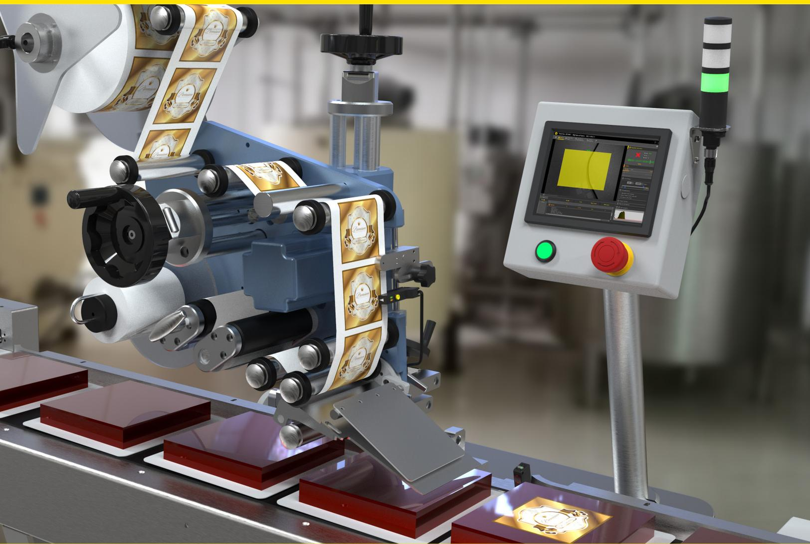
Banner Engineering offers a wide variety of industrial automation components that are ideal for use on labelling equipment including safety, indication and sensors. The SLE5 High Speed Optical Label Sensor was designed to reliably detect either labels or their backing. The simple, one-button TEACH mode provides fast sensor commissioning, and the dovetail design facilitates tool-less installation directly on the dispensing ledge.
