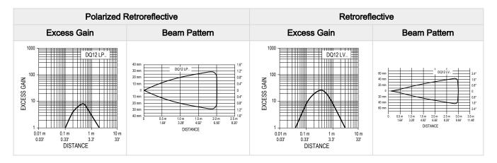
Fixed-field focus and spot sizes are typical. Performances are based on the use of a 90% reflectance white test card.\*
