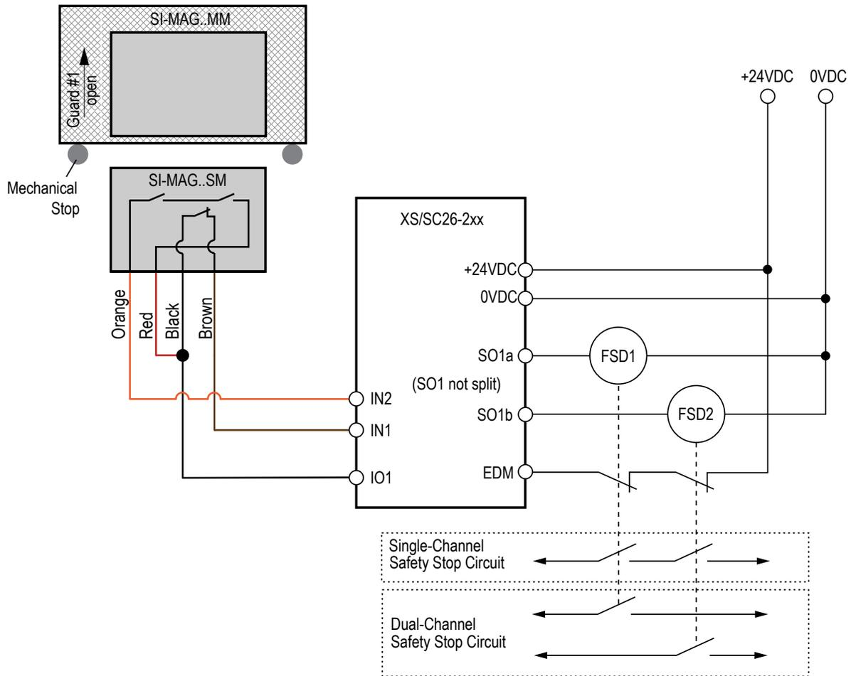
**IMPORTANT:** If the model number of the magnetic switch does not include a letter between the SI-MAG and the number, the orange wire shown is blue and the red wire is gray on older models.
