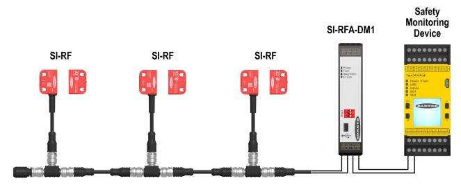
Figure 3. Connecting the SI-RF in series with a DM1 and monitoring device
