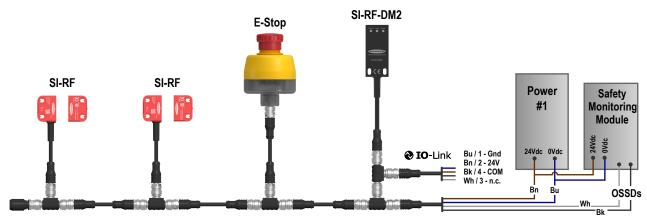
Figure 4. The SI-RFA-DM2 can be connected using a t-adapter (SI-RFA-TS) connected to a reset t-adapter (SI-RFA-TK)
