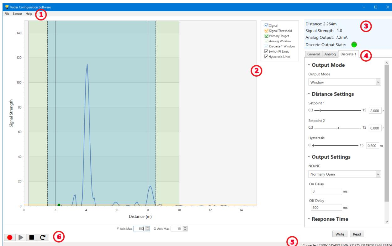
1. Navigation toolbar—Use this toolbar to connect to the sensor, to save or load a configuration, or to reset to factory defaults
