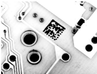
Figure 194. Data Matrix Code Directly Marked on PCB Surface by Using Laser Etching Technology
