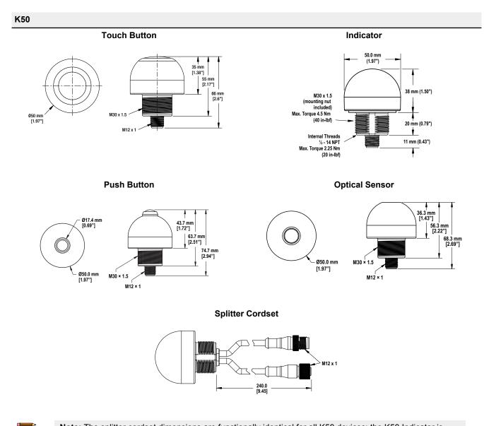
**Note:** The splitter cordset dimensions are functionally identical for all K50 devices; the K50 Indicator is shown.
