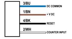
Figure 34. Wiring diagram for counter increment-decrement
