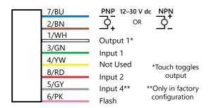
When configuring a 5-Wire K50 Pro Touch device to use two outputs, the Three State Advanced Control Device Logic Mode has two device states that are toggled by a single input wire.
