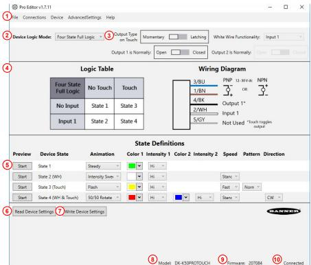
Figure 5. Pro Editor Configuration Navigation - K50 Pro Touch Shown **Tower Light Devices**
