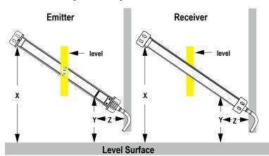
Figure 24. For angled or horizontal installations
