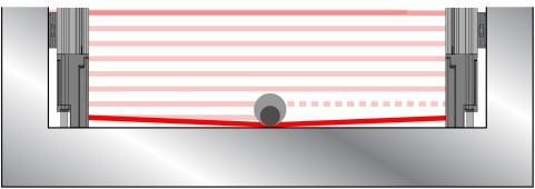
For 0.1 m to 3 m (4 in to 10 ft) Operating range: d = 0.13 m (5 in) For Operating range > 3 m (> 10 ft):  $d = 0.0437 \times R$  (m or ft)
