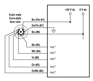
\*NOTE: Pins 2, 3, 4 and 5 either are not connected, or are paralleled to same color wire from the 8-pin receiver cable.
