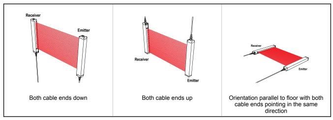
Figure 9. Examples of Incorrect Emitter/Receiver Orientation
