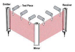
6. If the EZ-SCREEN LP Basic System passes all checks during the trip test, go on to Electrical Connections to the Guarded Machine on page 37.
