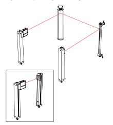
Figure 28. Corner Mirror Alignment
