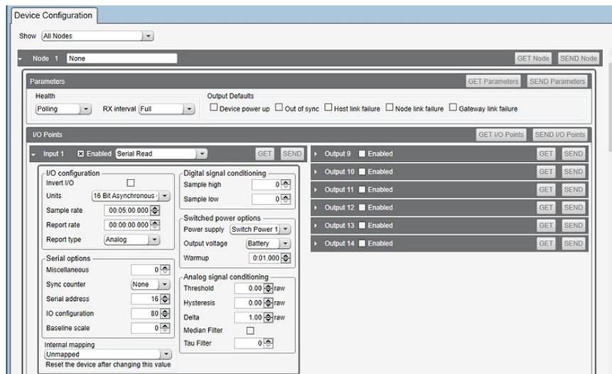
1. Go to the **Configuration > Device Configuration** screen.
