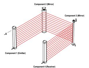
Figure 14. Corner Mirror Alignment
