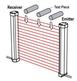
4. During each pass, while the test piece is interrupting the defined area, at least one Zone indicator must be red. The red Zone indicator must change with the position of the test piece within the defined area.
