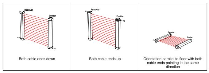
Figure 7. Examples of Incorrect Emitter/Receiver Orientation
