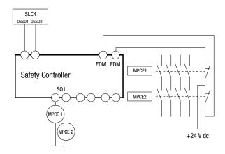
Single-channel EDM used to monitor both MPCE feedback signals. If one or both channels do not close, the system enters a lockout mode.
