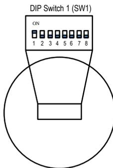
**Input channel select**—Use switch positions 1 through 6 on SW1, to select the channel that would be used to operate the audible module. Switch positions 7 and 8 are not used.
