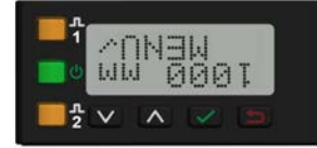
Figure 23. LE550 Inverted Display Orientation
