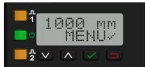
Figure 2. LE550 Display in Run Mode
