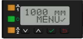
Figure 22. LE550 Normal Display Orientation
