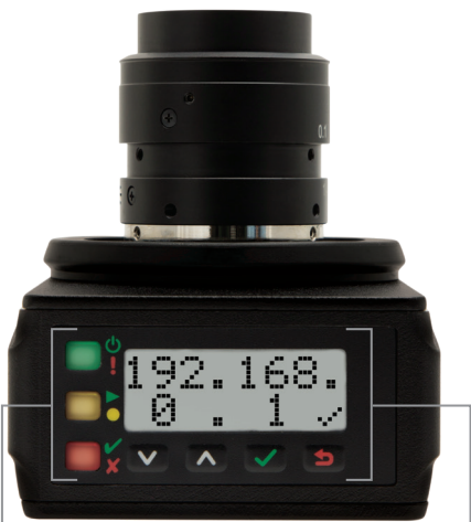
Bright LED indicators to easily view camera status Two-line, eight-character display and push buttons for troubleshooting and viewing camera status • Perform product change or trigger • Troubleshoot and clear errors • Change or view IP address, MAC address, or Ethernet speed • View firmware, focus number or status
