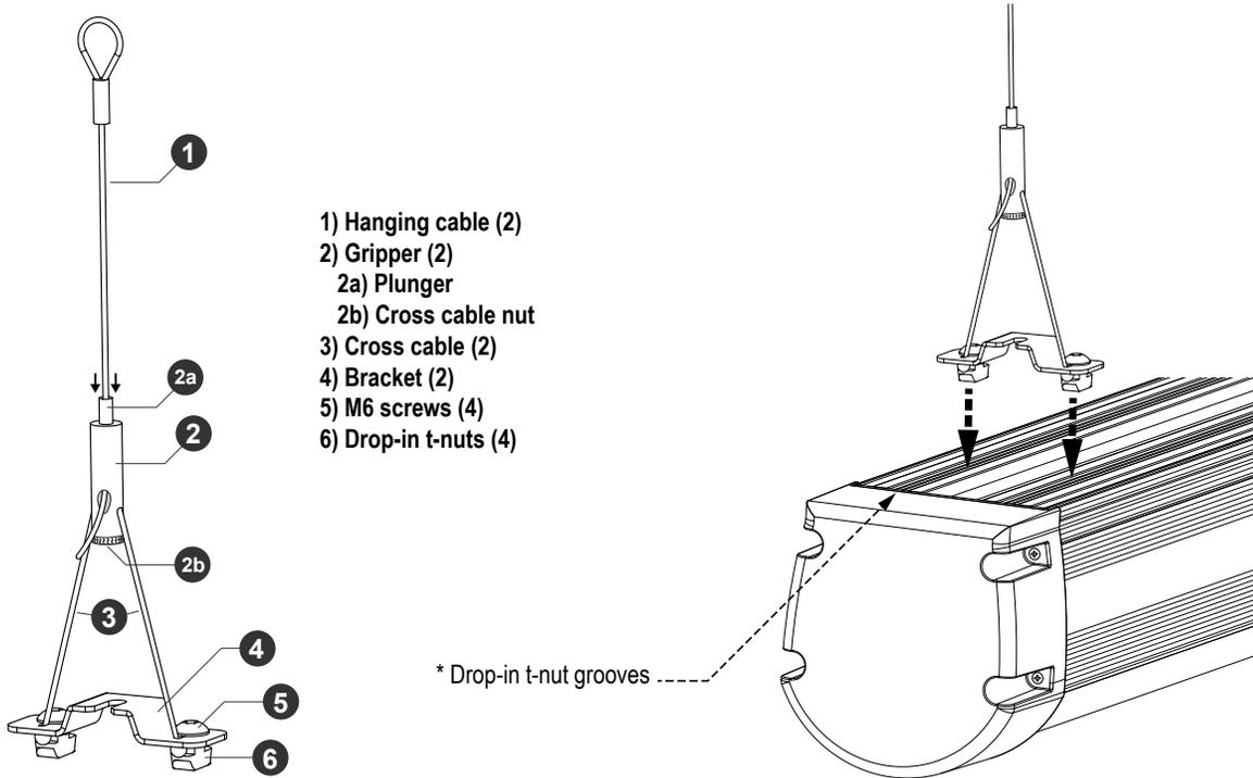
When feeding the cable through the gripper, allow at least one inch of cable beyond the gripper. Do not feed any excess cable into the light housing. To adjust the gripper position:
