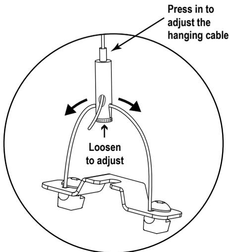
Drop-in t-nuts are automatically secured inside the grooves when they are tightened.
