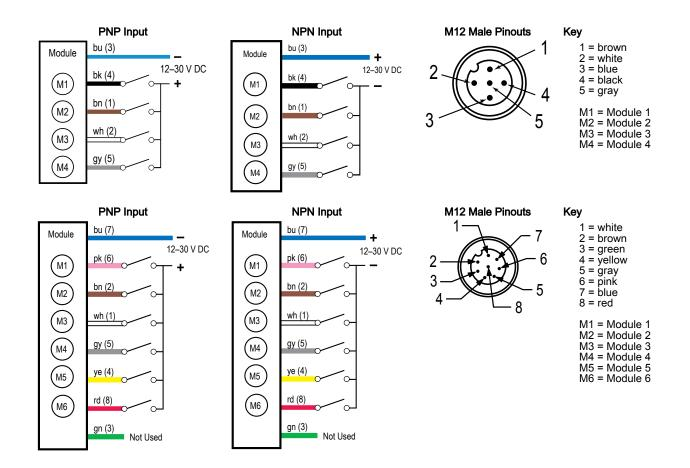
NOTE: Models SG-TL70-ALM and SG-TL70-ALMC are not compatible with NPN input wiring.
