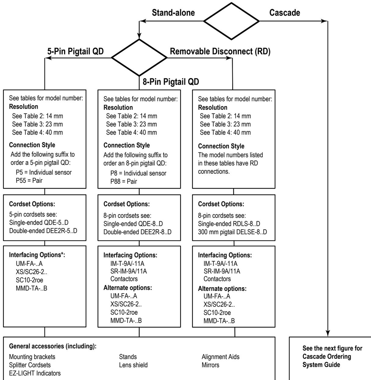
\* 5-pin models must be interfaced with a self-checking safety module, safety controller, or safety PLC/PES that conforms to the level of performance required by the risk assessment (such as Control Reliability and/or ISO13849-1 Categories 3 or 4 and PL d or e).
