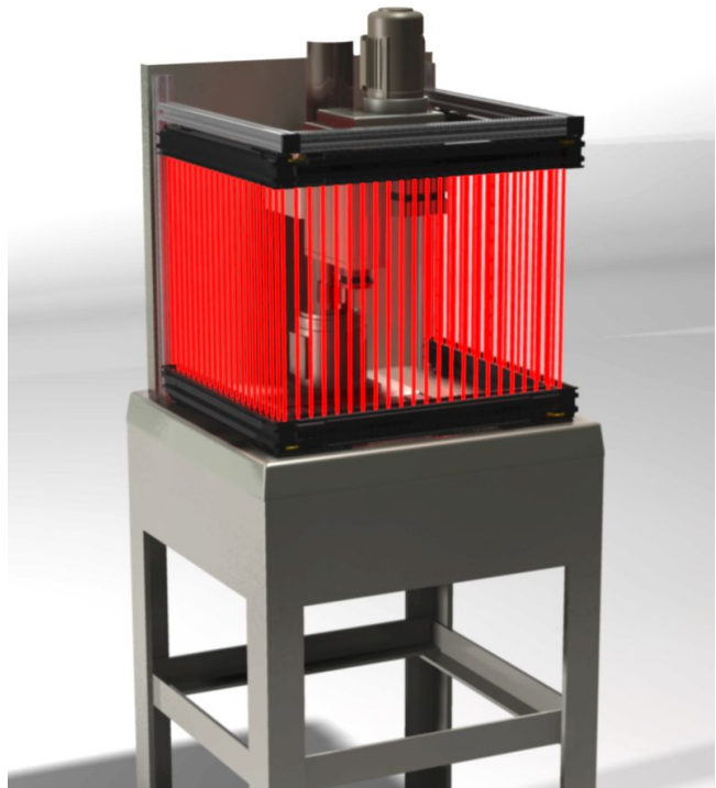
Figure 50. Cascaded light screens guarding a u-shaped cell
