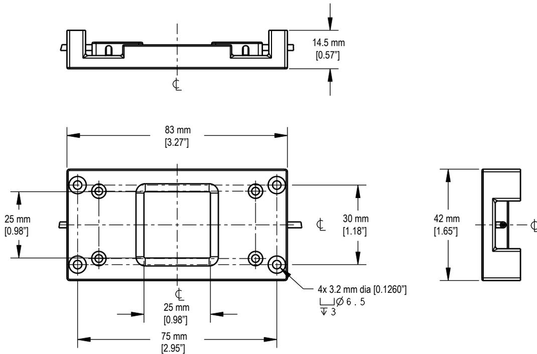
Figure 10. PFCVA-34X25-S and PFCVA-34X25-E
