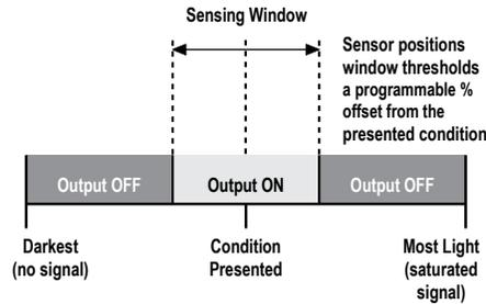
Output ON and OFF conditions can be reversed using the LO/DO switch.
