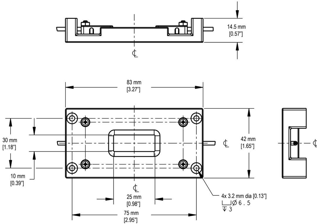
Figure 9. PFCVA-25X25-S and PFCVA-25X25-E
