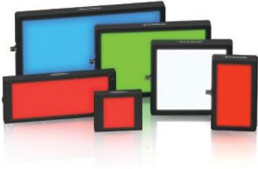
A backlight provides even bright lighting by placing the backlight behind the target and aiming it directly towards the camera. The resulting silhouette can be inspected for proper size and shape.
