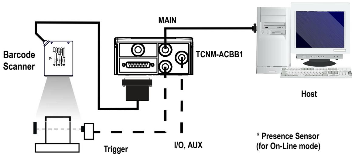
Figure 1. Barcode scanner in a standalone layout
