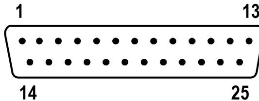
Figure 2. 25-pin male D-sub connector
