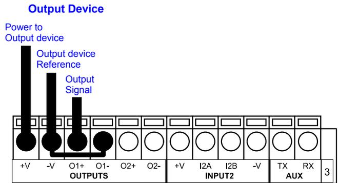
Figure 28. Open Collector Output Using Barcode Scanner Power
