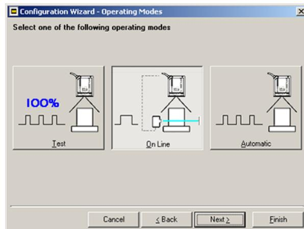
On Line operating mode requires the reader to be connected to an External Trigger/Presence Sensor using I1A and I1B inputs.
