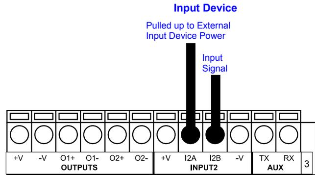
Figure 26. NPN Input 2 Using External Power
