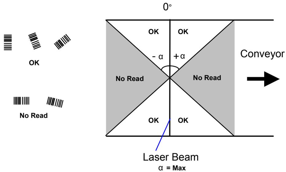
Figure 37. Reading Zones with  $\alpha$  Max
