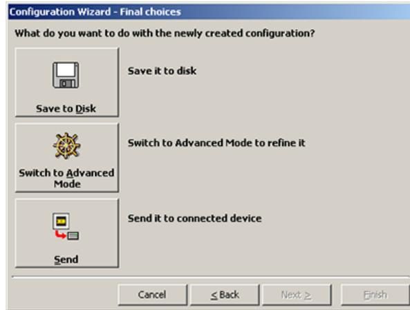
3. After sending the configuration to the scanner, click Next. You have completed the configuration process. Click Finish.
