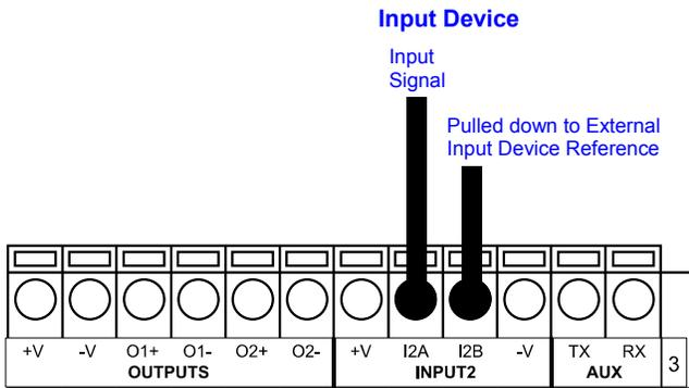
Figure 25. PNP Input 2 Using External Power
