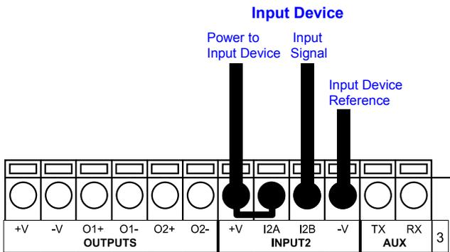
Figure 23. PNP Input 2 Using Barcode Scanner Power
