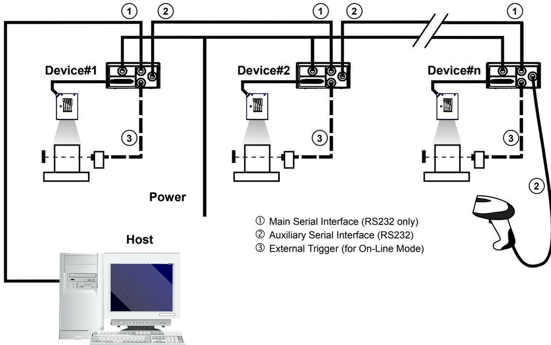
Figure 32. Pass-Through Layout
