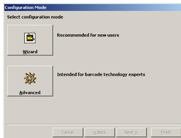
The Wizard option is advised for rapid configuration or new users because it shows a step-by-step scanner configuration.
