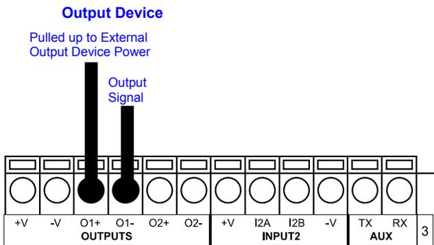
Figure 29. Open Emitter Output Using External Power
