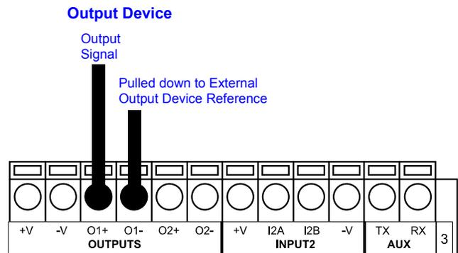
Figure 30. Open Collector Output Using External Power
