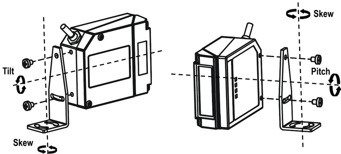
Figure 3. Positioning with Mounting Bracket at 10° Angle
