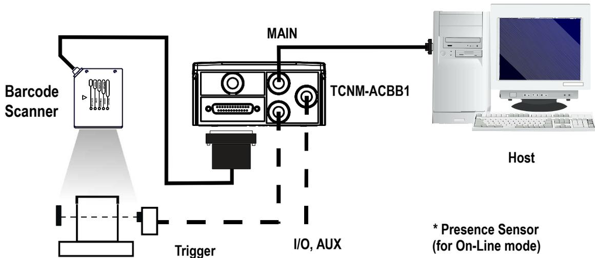
Figure 8. Barcode scanner in a standalone layout
