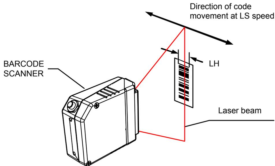
Figure 38. "Step-Ladder" Scanning Mode
