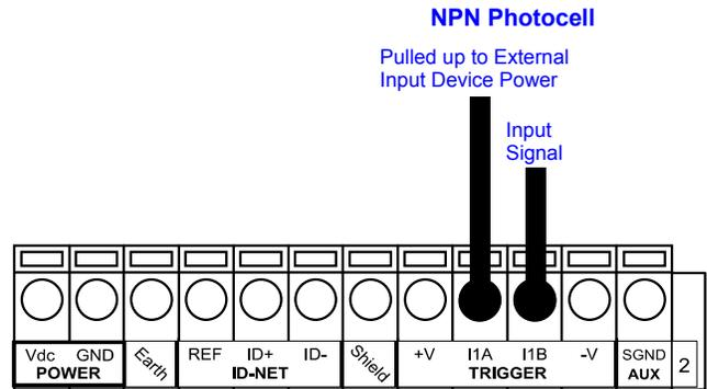
Figure 22. NPN External Trigger Using External Power
