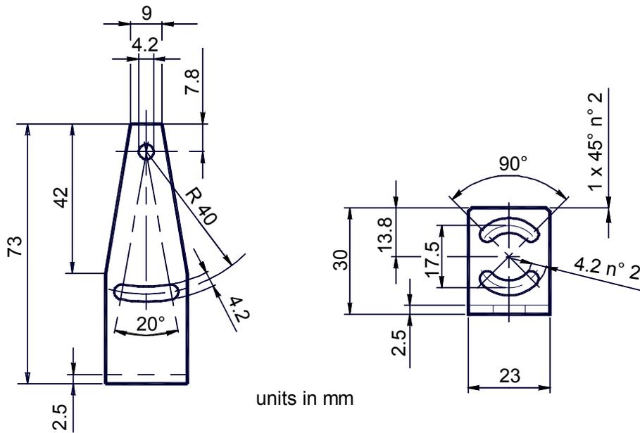
Figure 2. Mounting Bracket Overall Dimensions
