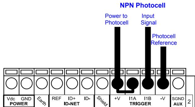
Figure 20. NPN External Trigger Using Barcode Scanner Power
