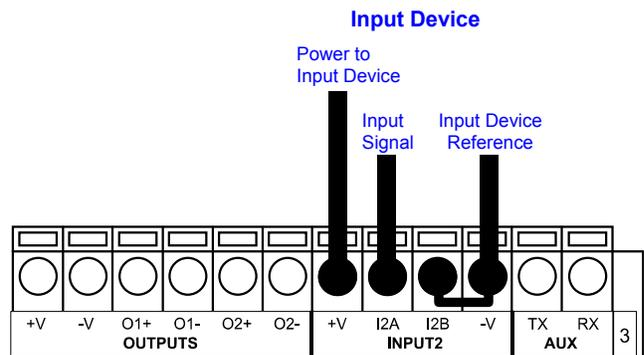
Figure 24. NPN Input 2 Using Barcode Scanner Power
