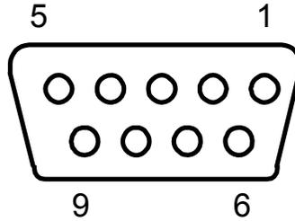
Figure 17. 9-pin female connector
