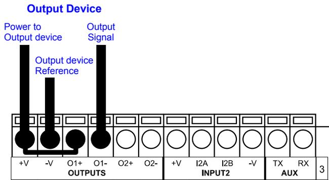
Figure 27. Open Emitter Output Using Barcode Scanner Power
