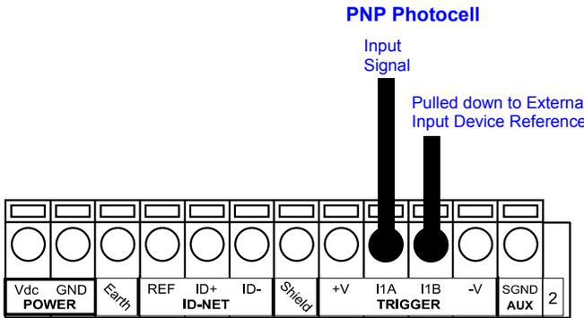
Figure 21. PNP External Trigger Using External Power
