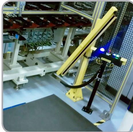
*Lithium ion battery cells are manufactured for installation in hybrid electric cars. Banner's Run Bar safety product was modified to provide operator guidance in a battery assembly workstation.*
