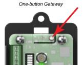
The LEDs flash alternately when the Gateway is in binding mode. Any Node entering binding mode will bind to this Gateway.
