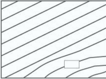
Baseline magnetic field with slight disturbances caused by permanent ferrous-metal objects within or near the sensor.
