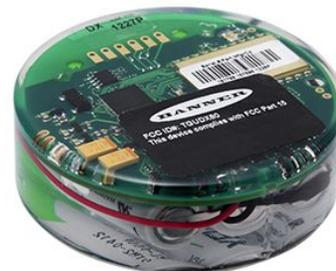
Do not open this device. This M-GAGE ships from the factory sealed and does not contain any serviceable parts. Opening this M-GAGE invalidates the manufacturer's warranty.
