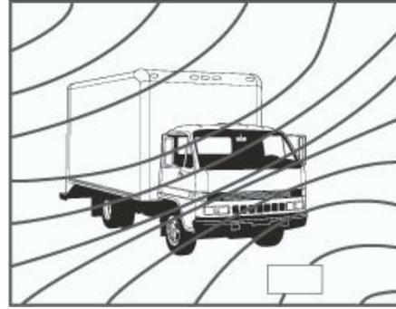
After a large object is introduced, the magnetic field changes. The sensor detects the changes in the field's strength and orientation between the ambient field and the field produced by a large metal object. If the differential is greater than the sensitivity threshold, the device reports a change of state.
