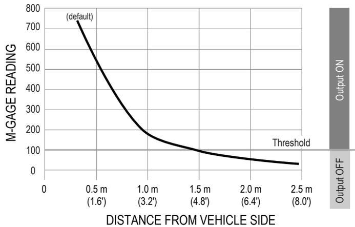
M-GAGE Reading when installed underground.
