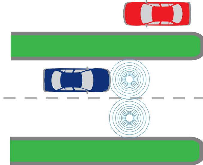
When the sensor is positioned in the middle of the traffic lane, it can be configured to a threshold level to detect vehicles only in the lane of interest. This is known as lane separation. A threshold level also aids the sensor in vehicle separation – detecting a break between the back bumper of a leading vehicle and the front bumper of the next vehicle. With proper placement and configuration, the M-GAGE can achieve vehicle separation with distances of 24 inches or less.
