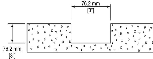
3. Verify all surfaces inside and near the hole are free of debris, warm (consult sealer manufacturer data for temperature threshold data), and thoroughly dry.
