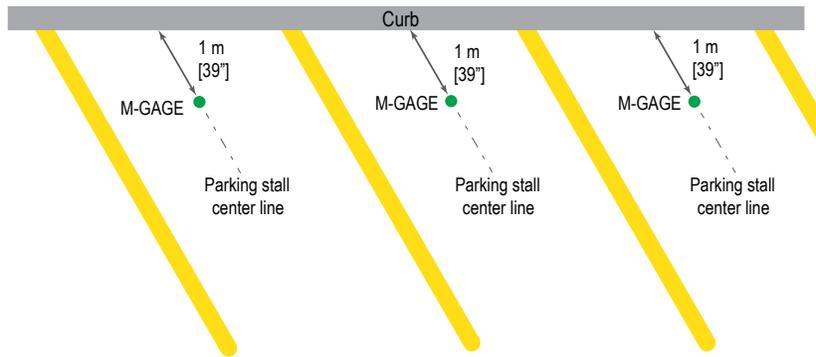
Optimum M-GAGE placement for parallel parking stalls
