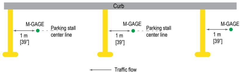
*Optimum M-GAGE placement for traffic detection*
