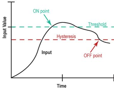
In the example shown, the input is considered on at 15 mA. To consider the input off at 13 mA, set the hysteresis to 2 mA. The input will be considered off when the value is 2 mA less than the threshold. Setting threshold and hysteresis points prevents inputs from oscillating between 'on' and 'off' when the input remains close to the threshold point.
