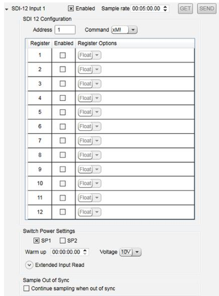
1. Select the **Enable** checkbox to enable the SDI-12 input.
