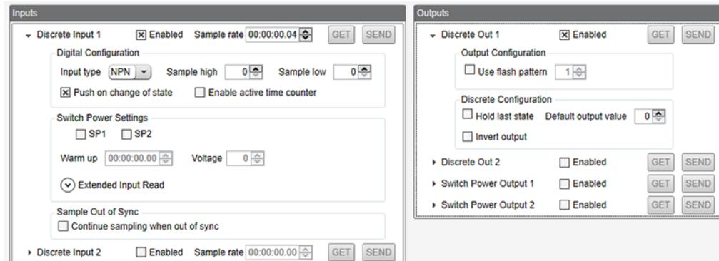
Select the device you want to configure by using the drop-down list to select the device address. Click **GET all parameters and IO** to retrieve any existing configuration data from the device.
