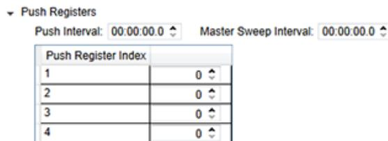
Up to four push registers may be defined for each MultiHop radio. For most applications, input registers are mapped to the push registers, but other registers may be configured as push registers, such as the battery read voltage. To configure a register as a push register:
