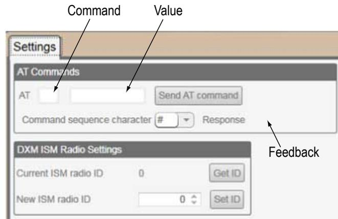
To assign a **New ISM radio ID** to a MultiHop radio within a DXM Controller, enter the new radio id and click **Set ID**.
