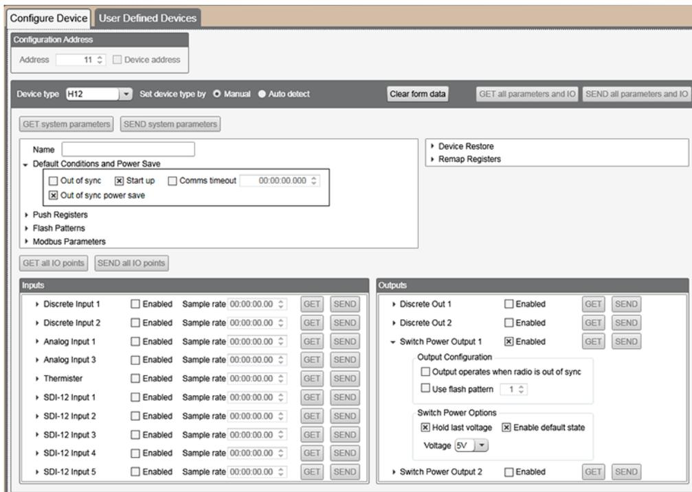
1. On the **Configuration > Configure Device** screen, enter the ID of the MultiHop radio that will be assigned a continuous power output and click **GET all parameters and I/O**.
