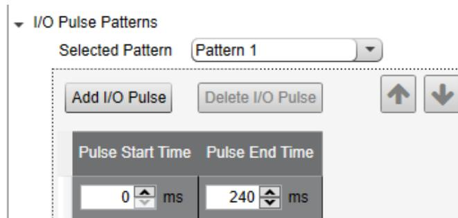
Define **I/O Pulse Patterns** by selecting specific timeslots to turn the output on or off. Although the pulse pattern was originally designed to turn on and off an indicator light, the pulse pattern can be set for any discrete output or switch power. Users may configure up to four different patterns per radio device. In the example shown, Pattern 1 is configured to turn on for the first 240 milliseconds within a 1280 millisecond range.
