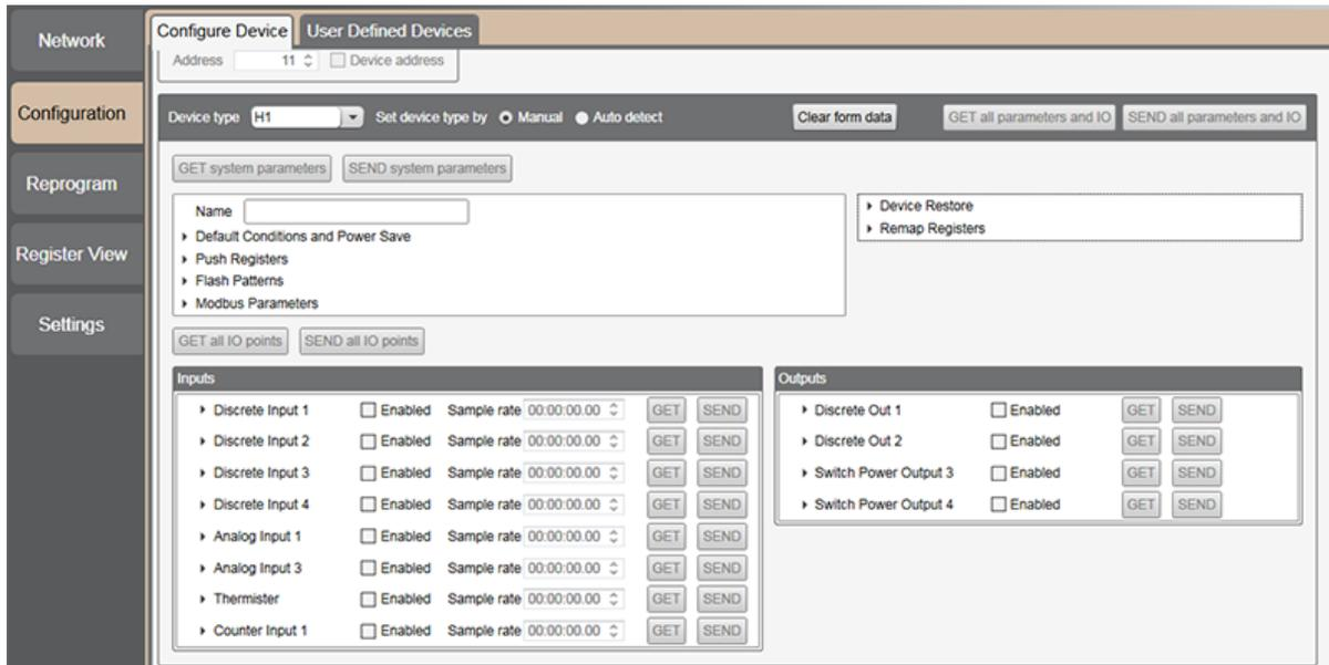
**Manual Mode**—Select the **Manual Mode** checkbox and select the **Device Type** from the drop-down list. Selectable device types are:
