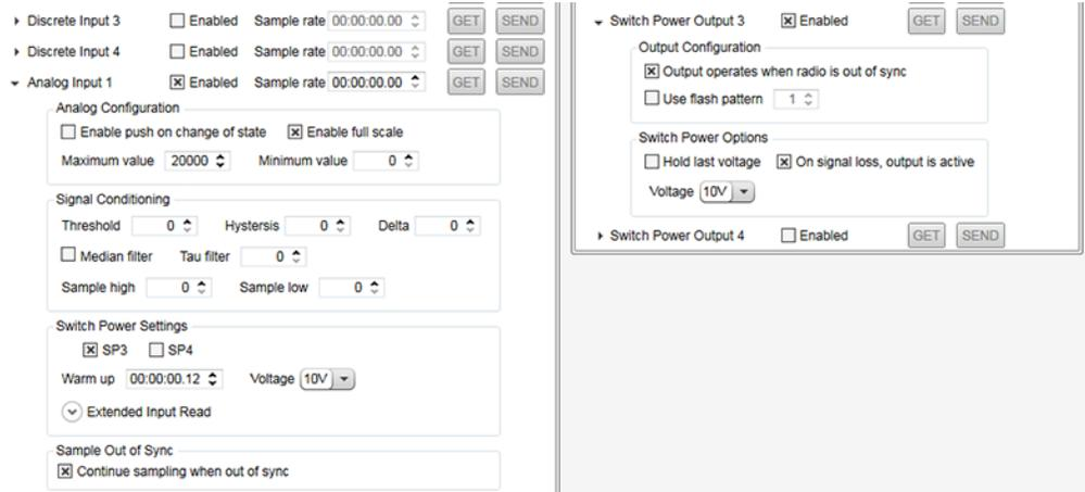
1. Go to the Analog IN 1 section of the **Configuration > Configure Device** screen and select the **Enabled** checkbox.
