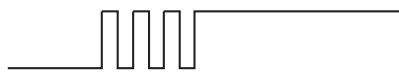
Without a debounce filter, the signal is interpreted to change state multiple times.
