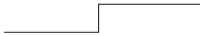
With a debounce filter, the signal is interpreted to change state only once.
