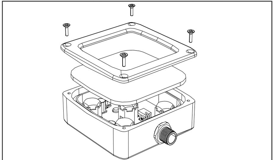
Figure 1. Installing the replacement window on the light
