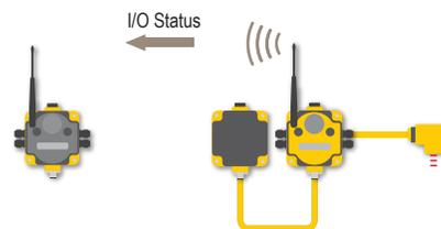
**Re-link Count** The re-link count is the number of completed polling messages the Gateway receives from a Node before a lost RF link is considered re-established and normal operation resumes.
