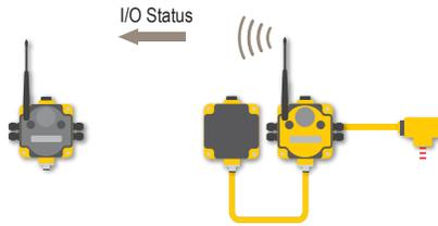
**Report Type** Select from discrete or analog format reporting types. Analog data requires sixteen bits while discrete data uses only one bit per I/O point. Selecting double from the list uses two consecutive registers, each consisting of sixteen bits.
