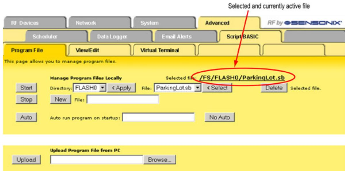
When a file is selected, the filename.sb is shown as a link above the Select button. Click on this link to download the file to the PC. To upload a file from the PC, use the Browse and Upload buttons. Use the following buttons to create and manipulate files.
