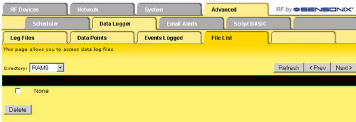
**Delete** To delete the files, select the checkbox for the unwanted file then click the Delete button.
