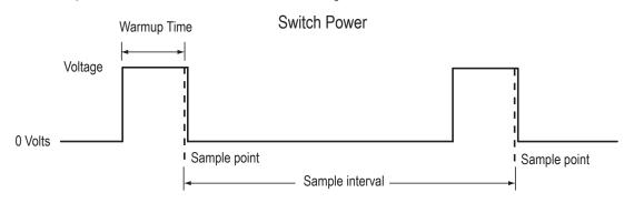
Efficient power management technology enables the FlexPower battery system to briefly step up the switched power voltage to activate the low-power MINI-BEAM® sensor, which is optimized for low duty cycle pulse operation. Once activated, the input reads the sensor then the switched power shuts off to prolong battery life, operating the MINI-BEAM in short pulses rather than continuously.
