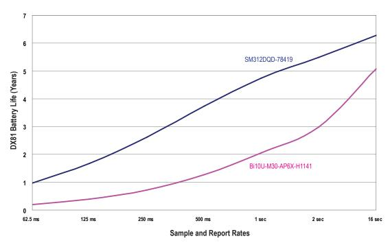
For each sensor characterized, a boost voltage and warmup time was specified. The sample and reports rates were varied to calculate the estimated battery life. For example, a Banner Optical sensor, model SM312DQD-78419, set to a boost voltage of 5 volts, a warm-up time of 4 milliseconds, and a sample and report rate of 16 seconds, should have a battery life of just over 6 years.
