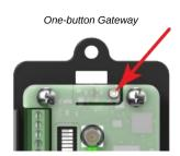
The LEDs flash alternately when the Gateway is in binding mode. Any Node entering binding mode will bind to this Gateway.
