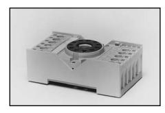
The RS-11 is supplied with a coding ring and pin (see diagram at right). This allows a MAXI-AMP to be keyed to fit only its own 11-pin socket. The pin is installed in one of the eleven slots in the RS-11, and the notch in the ring is aligned to slip over the pin. When the MAXI-AMP is removed from the RS-11, the coding ring stays with the MAXI-AMP base, while the coding pin remains in the socket.
