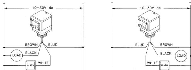
The Bi-Modal™ output of OMNI-BEAM dc power blocks is wired for **current sinking** (NPN) operation (100mA max.) by connecting the BROWN supply wire to +V dc, and the BLUE wire to dc common.
