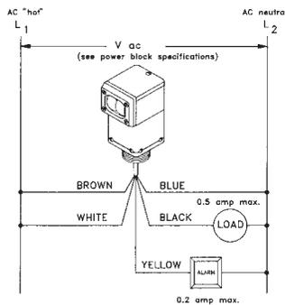
\*Note that when standard OMNI-BEAM power blocks are used with the OSBFAC, the power block ALARM output functions as a second output that exactly follows the action of the main output. The capacity of this second output is 100mA max. (for dc-powered power blocks) and 200mA
