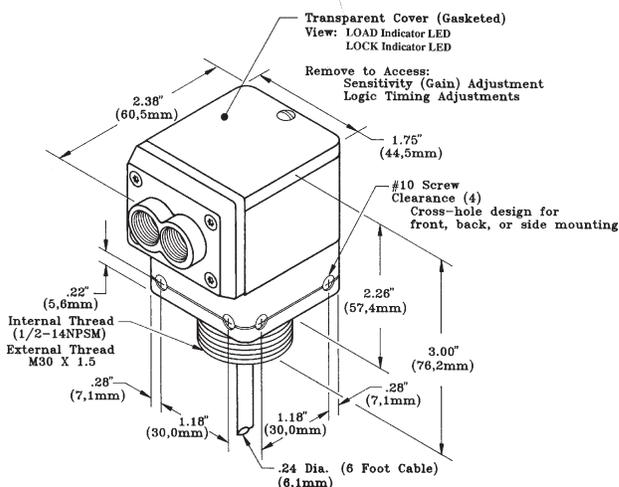
\*Standard ac power block is .88" taller in height; overall height of OSBFAC sensor head with an ac power block attached is 3.88".
