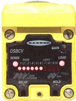
Banner’s exclusive D.A.T.A. feature warns of marginal sensing conditions, usually before a sensing failure occurs, by flashing one or more lights in its multiple-LED array, and by sending a warning signal to the system logic controller (or directly to an audible or visual alarm). The chart below describes the meanings of the possible signals.
