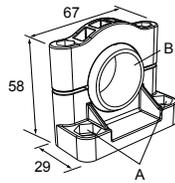
Hole center spacing: A=ø 50.8
