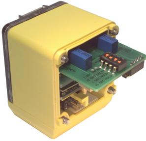
Timing logic may be added at any time, using one of three timing delay and pulse logic modules. Installation is simple and quick; the logic modules simply slide into the sensor head. Program them for timing functions and ranges via four DIP switches; each module includes easily accessible 15-turn clutched potentiometers for accurate timing adjustments.
