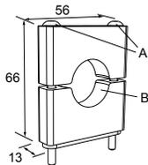
Hole center spacing: A=ø 45
