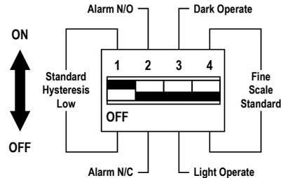
Figure 2. OMNI-BEAM DIP switch configuration
