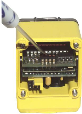
Figure 1. OMNI-BEAM DIP switch location
