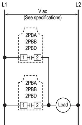
Figure 4. 2-Wire MULTI-BEAMs in Parallel
