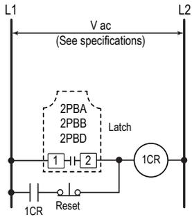
Figure 7. Photoelectric Latch with Manual Reset
