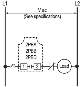
Figure 5. 2-Wire MULTI-BEAM with Series Contacts
