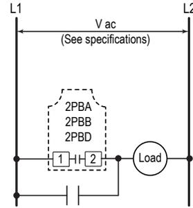
Figure 6. 2-Wire MULTI-BEAM with Parallel Contacts
