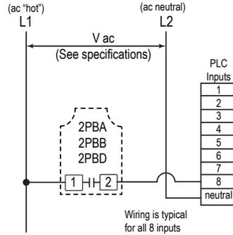
Figure 8. 2-Wire MULTI-BEAM to Programmable Logic Controller (PLC)
