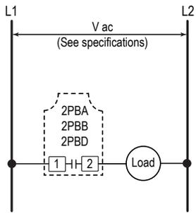
Figure 3. Basic Wiring of 2-Wire MULTI-BEAM
