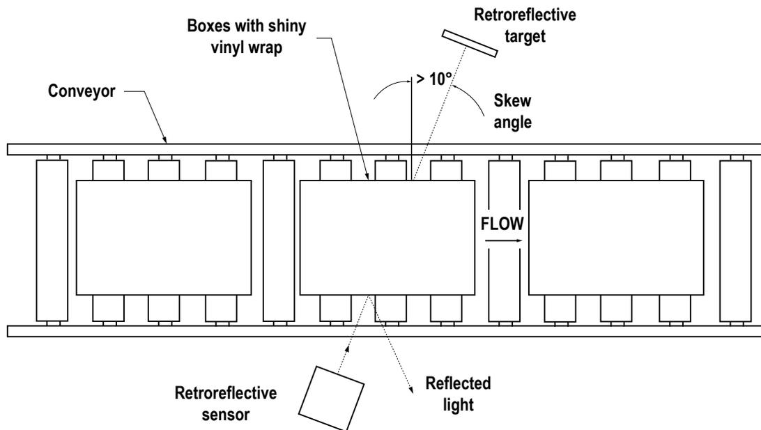
Proper operation of retroreflective mode sensors requires that they be mounted securely and aligned properly. Excessive movement or vibration can result in intermittent or false operation caused by loss of alignment to the retroreflective target. Banner offers a variety of two- and three-axis mounting brackets for use with MULTI-BEAM sensors. See [www.bannerengineering.com](http://www.bannerengineering.com) for bracket information.
