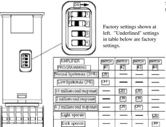
NOTE: the LOW hysteresis setting should be used only when all sensing conditions remain stable. "Buzzing" of the output (in ON/OFF and LIMIT operation) or false outputs (in DELAY, ONE-SHOT, or LATCH operation) may occur if sensing variables (e.g.- web flutter) result in optical contrast approaching unity.
