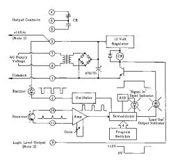
NOTE #3: pin #9 of CR3 model may be connected directly to the AUXILIARY input of a MAXI-AMP or Banner M Series module. It may also serve as the input to Banner CL series MAXI-AMPs or to Banner Plug Logic modules.
