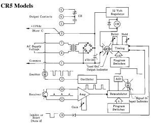
**NOTE #1:** power is available at pins #3 (+) and #1 (-) for an external 10 to 30V dc device (see hookup example, page 4). Current available is 40 mA at 120V ac (240V ac) line level; 30mA at 105V ac (210V ac) line level. Alternately, the module may be powered by 12 to 28V dc at pins #3 (+) and #1 (-). Do not connect ac voltage if using external dc power.
