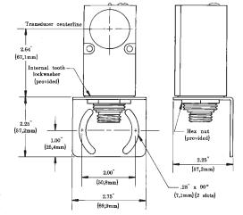
tility in mounting and orientation. The sensor mounts to the bracket by its threaded base, using a jam nut and lockwasher (both included). The bracket material is 11-gauge zinc-plated steel. The curved mounting slots have clearance for 1/4" screws.
