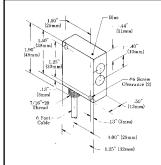
Model SP300L is a remote retroreflective sensor with the same rugged design as the SP300EL/RL, described above. Its useable range is from 6 inches to 15 feet (0,2 to 4,5m) using the model BRT-3 retroreflector.
