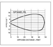
lenses to increase range. These sensors should also be used at short ranges for their high excess gain or to avoid optical "crosstalk" in situations which require several pairs to be mounted adjacent to one another.
