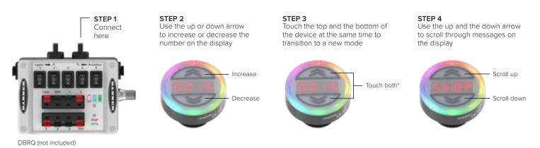
\*The device will transition between demo functions any time the top and bottom arrows are touched at the same time
