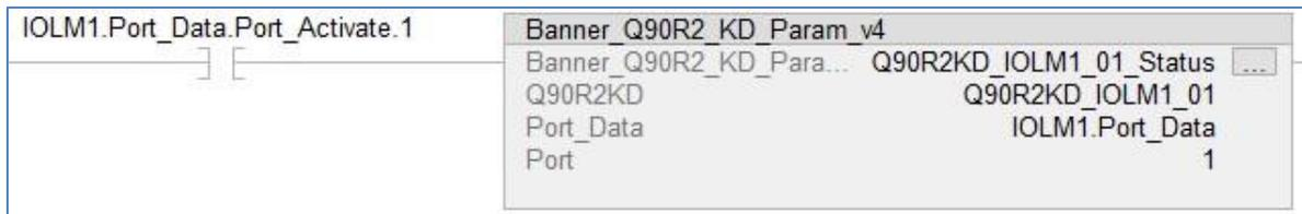
3. The Q90R2KD AOI is now linked to the IO-Link Master AOI. Add an Examine On instruction to the beginning of the ladder rung and tie it to the IO-Link Master AOI’s “Port Activate” bit corresponding to the port number to which the Q90R2KD is connected. In this example the Q90R2KD is on port 1 of the IO-Link Master named IOLM1, so the bit “IOLM1.Port\_Data.Port\_Activate.1” is used.
