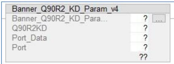
2. In the AOI, right-click on the question mark on the line labeled “Banner\_Q90R2\_KD\_Param\_v4”. Click New Tag. In this example, we’ll use the name “Q90R2KD\_IOLM1\_01\_Status”. The example naming convention accounts for this being a Q90R2KD sensor connected to IO-Link Master #1, port #1, in our program. More masters could be named IOLM2, IOLM3, and different sensors could be connected at other port numbers, etc.
