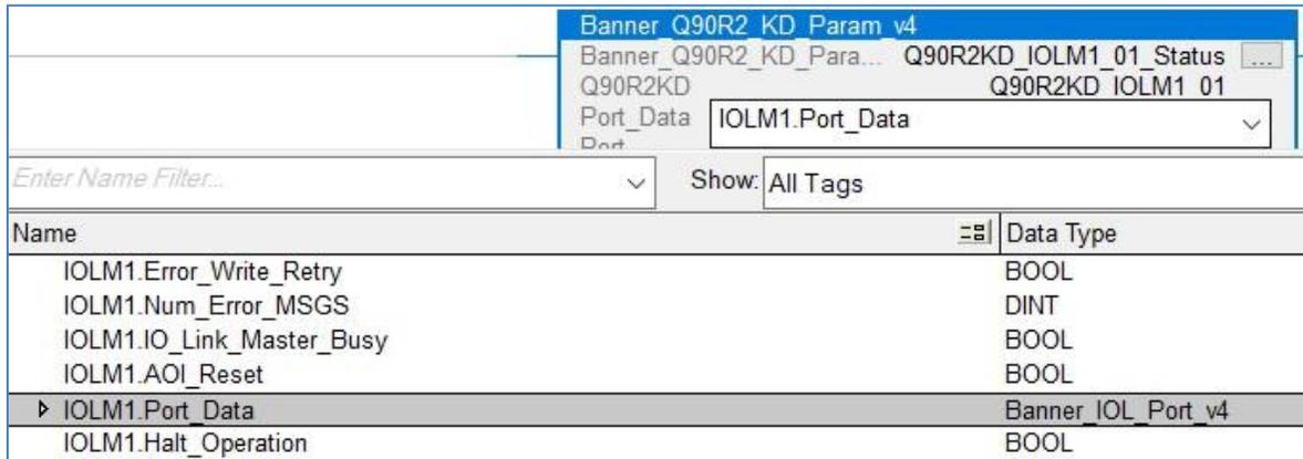
2. For the last line of the Q90R2KD AOI, “Port”, type in a number equal to the IO-Link Master port number to which the Q90R2KD is connected. In this example, the Q90R2KD is on port 1.
