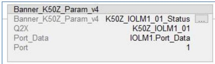
3. The K50Z AOI is now linked to the IO-Link Master AOI. Add an Examine On instruction to the beginning of the ladder rung and tie it to the IO-Link Master AOI's "Port Activate" bit corresponding to the port number to which the K50Z is connected. In this example the K50Z is on port 1 of the IO-Link Master named IOLM1, so the bit "IOLM1.Port\_Data.Port\_Activate.1" is used.
