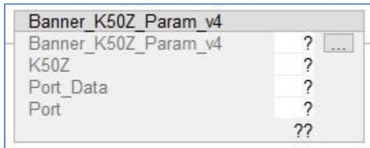
2. In the AOI, right-click on the question mark on the line labeled “Banner\_K50Z\_Param\_v4”. Click New Tag. In this example, we’ll use the name “K50Z\_IOLM1\_01\_Status”. The example naming convention accounts for this being a K50Z sensor connected to IO-Link Master #1, port #1, in our program. More masters could be named IOLM2, IOLM3, and different sensors could be connected at other port numbers, etc.
