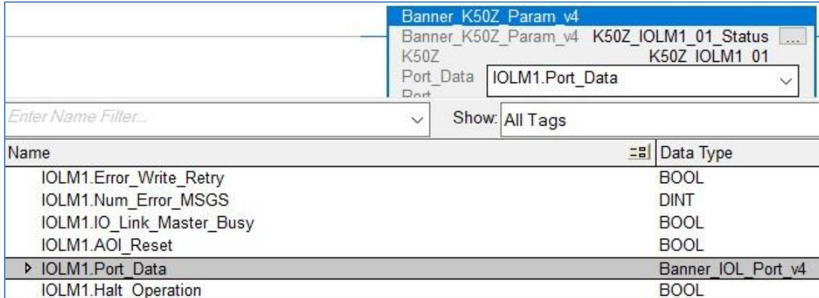
2. For the last line of the K50Z AOI, “Port”, type in a number equal to the IO-Link Master port number to which the K50Z is connected. In this example, the K50Z is on port 1.
