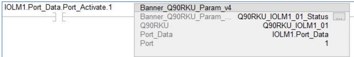
3. The Q90R KU AOI is now linked to the IO-Link Master AOI. Add an Examine On instruction to the beginning of the ladder rung and tie it to the IO-Link Master AOI’s “Port Activate” bit corresponding to the port number to which the Q90R KU is connected. In this example the Q90R KU is on port 1 of the IO-Link Master named IOLM1, so the bit “IOLM1.Port\_Data.Port\_Activate.1” is used.
