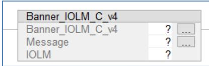
2. In the AOI, right-click on the question mark on the line labeled “Banner\_IOLM\_C\_v4”. Click New Tag. In this example, we’ll use the name “IOLM1\_Status”. The example naming convention accounts for this being the #1 IO-Link Master in our program. More masters could be named IOLM2, IOLM3, etc.
