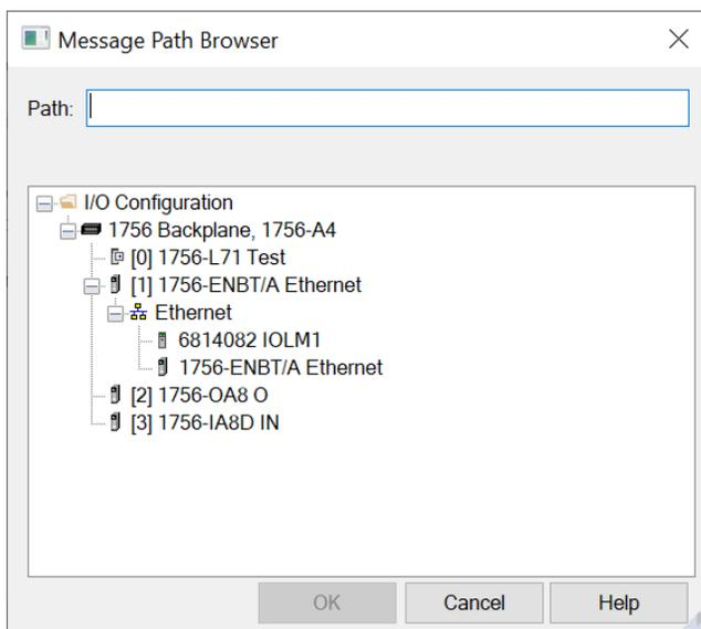
11. Now configure “Message\_Write”, setting up the Explicit Message that will handle the other half of the communications between the PLC and the IO-Link Master. Click on the “...” button at the far right of the “Message\_Write” line.
