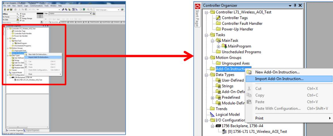
3. Navigate to the correct file location and select the AOI to be installed. In this example the "Banner\_IOLM\_T2\_v4.L5X" file will be selected. Click the Open button.
