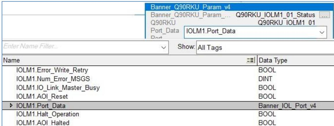
2. For the last line of the Q90R KU AOI, “Port\_Number”, type in a number equal to the IO-Link Master port number to which the Q90R KU is connected. In this example, the Q90R KU is on port 1.
