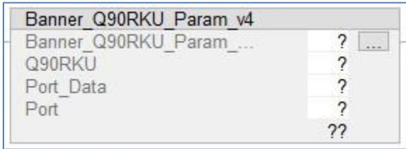
2. In the AOI, right-click on the question mark on the line labeled “Banner\_Q90RKU\_Param\_v4”. Click New Tag. In this example, we’ll use the name “Q90RKU\_IOLM1\_01\_Status”. The example naming convention accounts for this being a Q90RKU sensor connected to IO-Link Master #1, port #1, in our program. More masters could be named IOLM2, IOLM3, and different sensors could be connected at other port numbers, etc.
