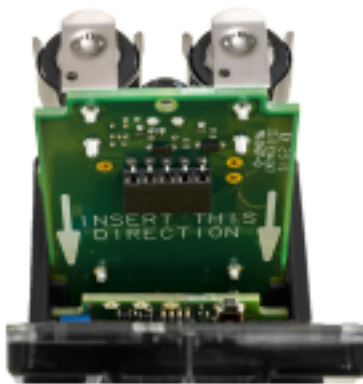
Figure 6. Q45 battery board
