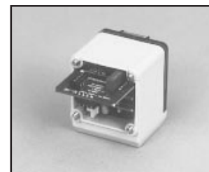
The OALM analog board slides easily in and out of the sensor head.
