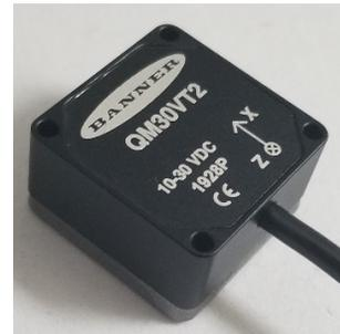
3. Screw the sensor to the bracket with the provided screws using a 2 mm Hex Allen wrench. The maximum torque for socket head screws is 0.5 N·m. Do not over tighten.
