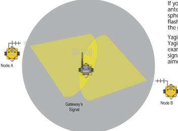
If you compare antenna radiation patterns to light, an omni antenna radiates a radio signal like a light bulb — evenly in a spherical pattern. A directional antenna radiates similar to a flashlight — focusing the signal only in one direction. The higher the gain, the more focused the beam becomes.
